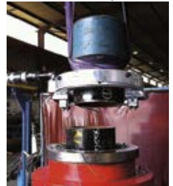
ECC can be inverted for cuts low to the wellhead
