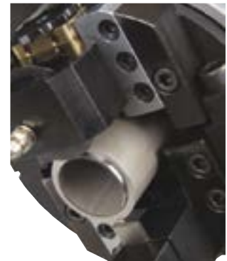
Wheel Cutting Module for FME Cutting
