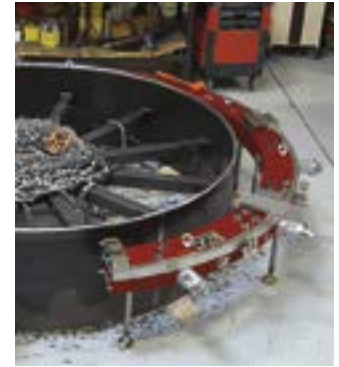
Four standard LDSF sizes cover 60-120in (DN1500-3000)
