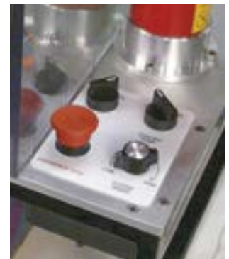
Controls are externally mounted and grouped together for convenience.
