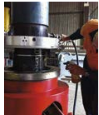
ECC can be inverted for cut lines close to the flange
