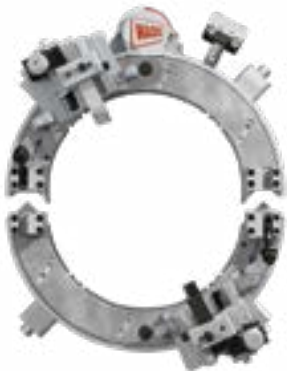
MDSF Split Frame unbolted for OD mounting
