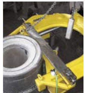
Goliath Saw shown on large diameter conductor
