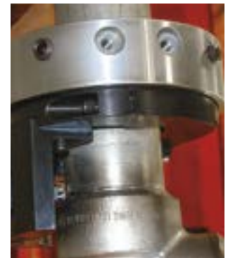
Axial Socket Weld Removal
